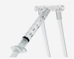
4. Make sure the tubing coming off the manifold is directed away from the foot pump:
