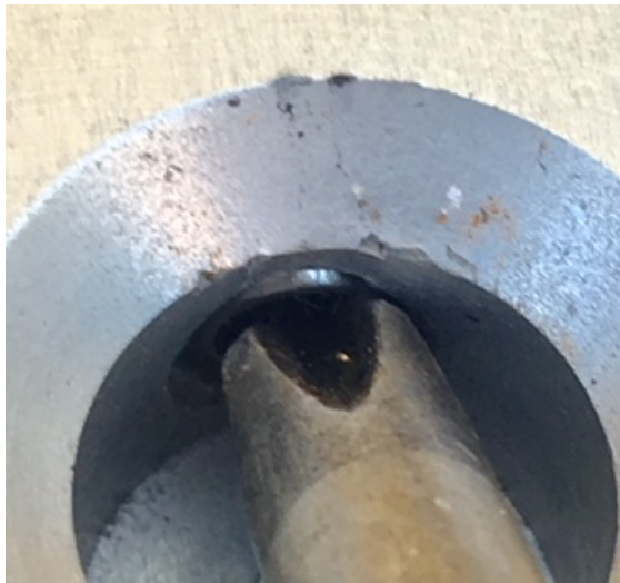
PUSH BEARING IN WITH A SCREWDRIVER
